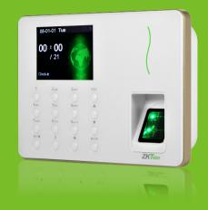
WL30 is Fingerprint Time & Attendance Terminal with Wi-Fi module. With Wi-Fi function, User needn't wire Ethernet cable, it supports hotspot mode and allow mobile APPs connection and check in/out and download record directly. It's associated with ZK new fingerprint reader, the operation remains stable under strong light source and high preciseness of verification of wet and rough fingers. It also has elegant design, it will start new stage of time attendance.
